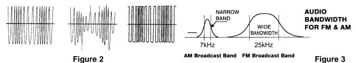
The standard broadcast band for FM was also designed to have an audio range up to 25,000 Hertz (Hertz = cycles per second). The standard AM broadcast band has only 7,000 Hertz band width (Figure 3). The FM band is therefore considered to be "High Fidelity" compared to the older AM band.
