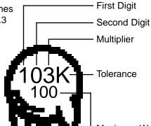
The letter M indicates a tolerance of  $\pm 20\%$ The letter K indicates a tolerance of  $\pm 10\%$
