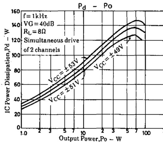
Fig.1 STK4231II Pd - Po ( $R_L = 8\Omega$ )
